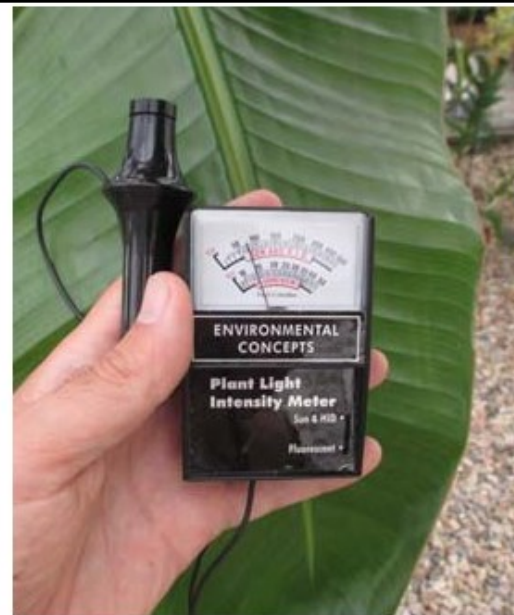
Growers use light meters such as this to measure the intensity of the sun near their orchids. Now cell phones can perform the same function.
